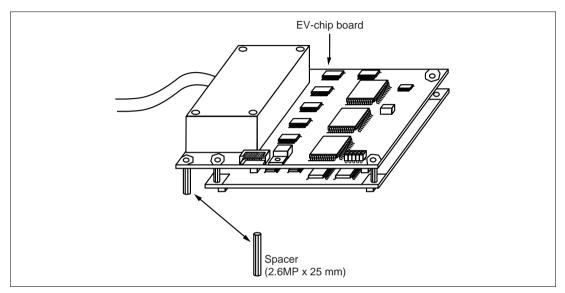
Figure 3 Exchanging the Spacer
